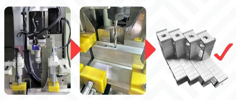
We have equipped our slicing and drilling machine with a high-precision and high-torque servo motor, enabling it to open tapping on profiles. This will allow you to perform your operations very quickly and precisely in your multiple operations.
