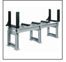
Loading and unloading roller table with containment vertical roll with adjustable width. Single module length is 2m. This model is compatible with bundle cutting, also equipped with trail to collect remaining and liquid
