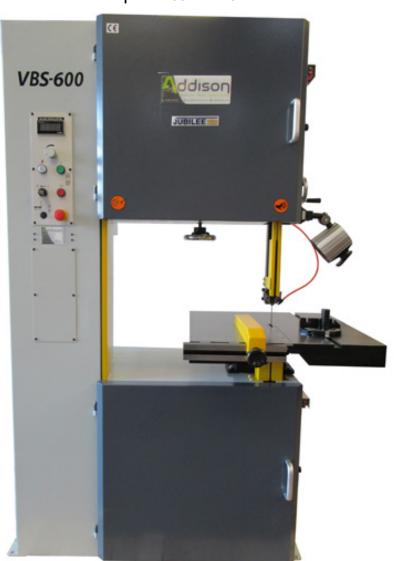
Digital display of the band speed Electric swarf blower Calibrated scale for band tension Option for oil mist lubrication Ontion for dust extraction
