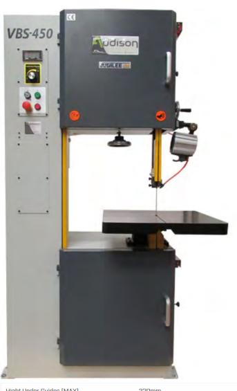
Digital display of the band speed Electric swarf blower Calibrated scale for band tension Option for oil mist lubrication Option for dust extraction
