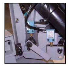
Adapter to synchronize roller table/machine (Optional)
