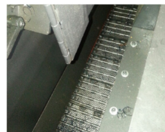
Automatic chip conveyor under saw blade directly
