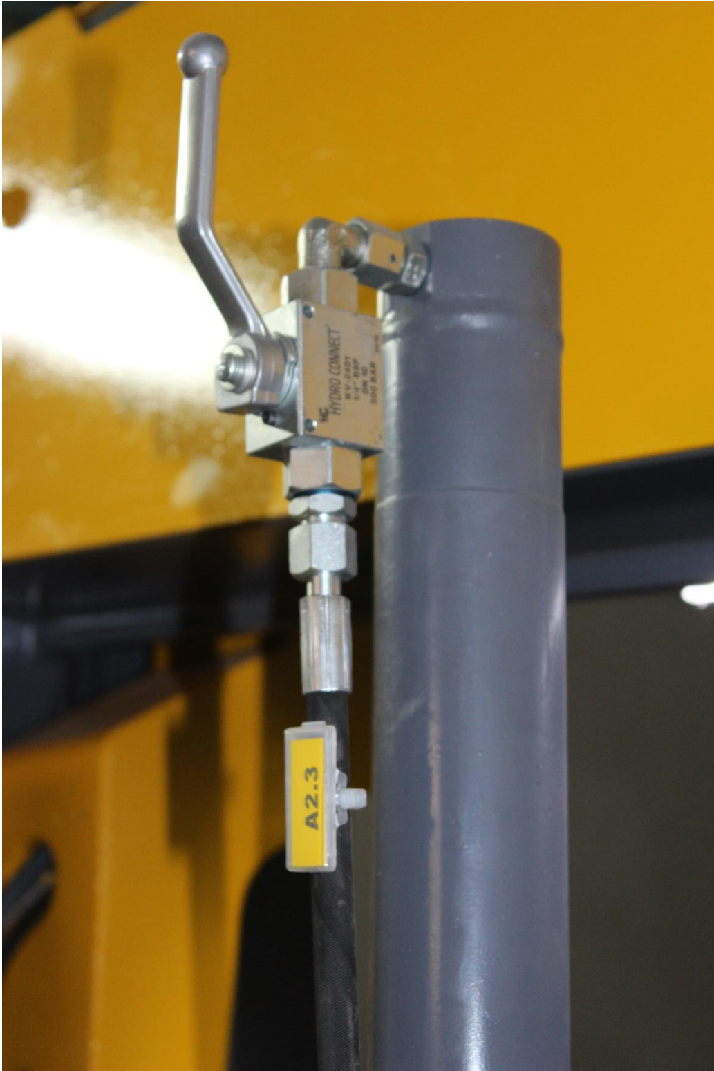
HYDRAULIC VALVE TO CLOSE/OPEN UPPER CLAMP
