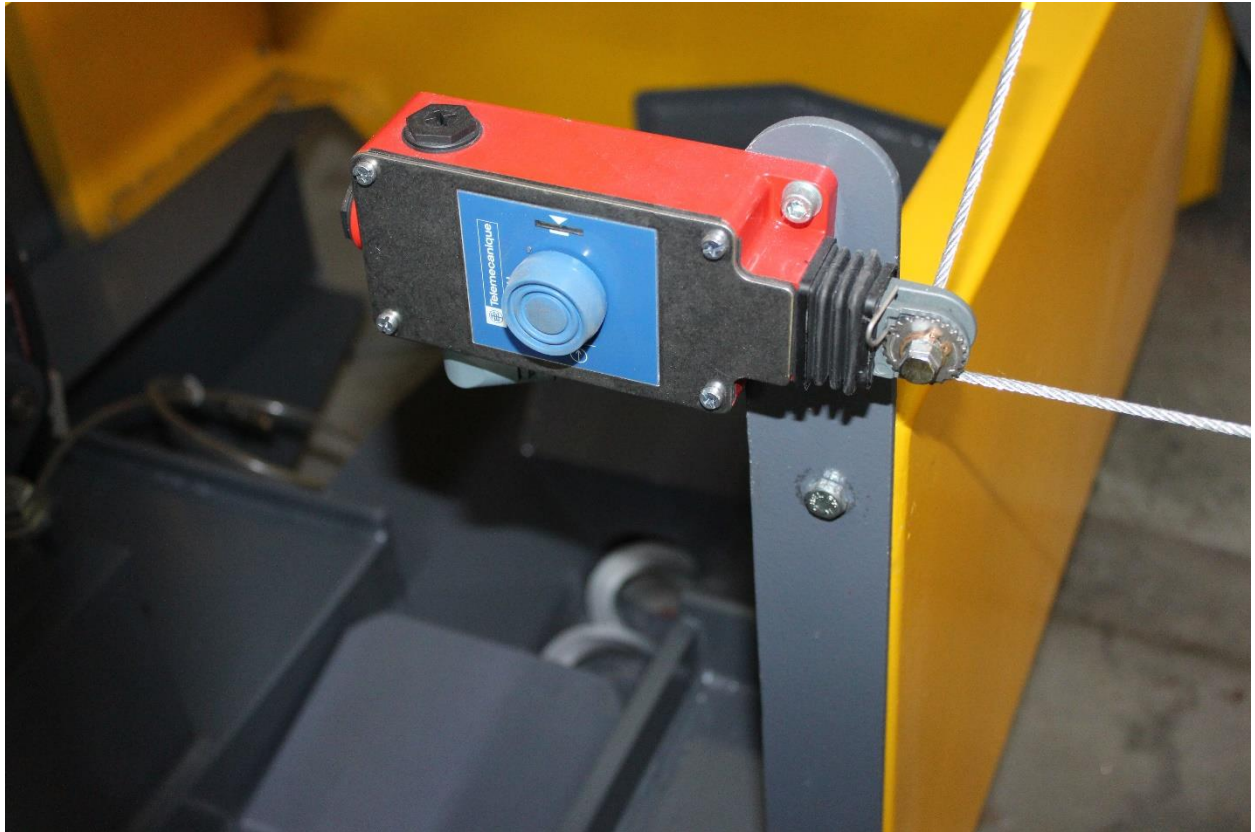
SAFETY WIRE WITH SWITCH
