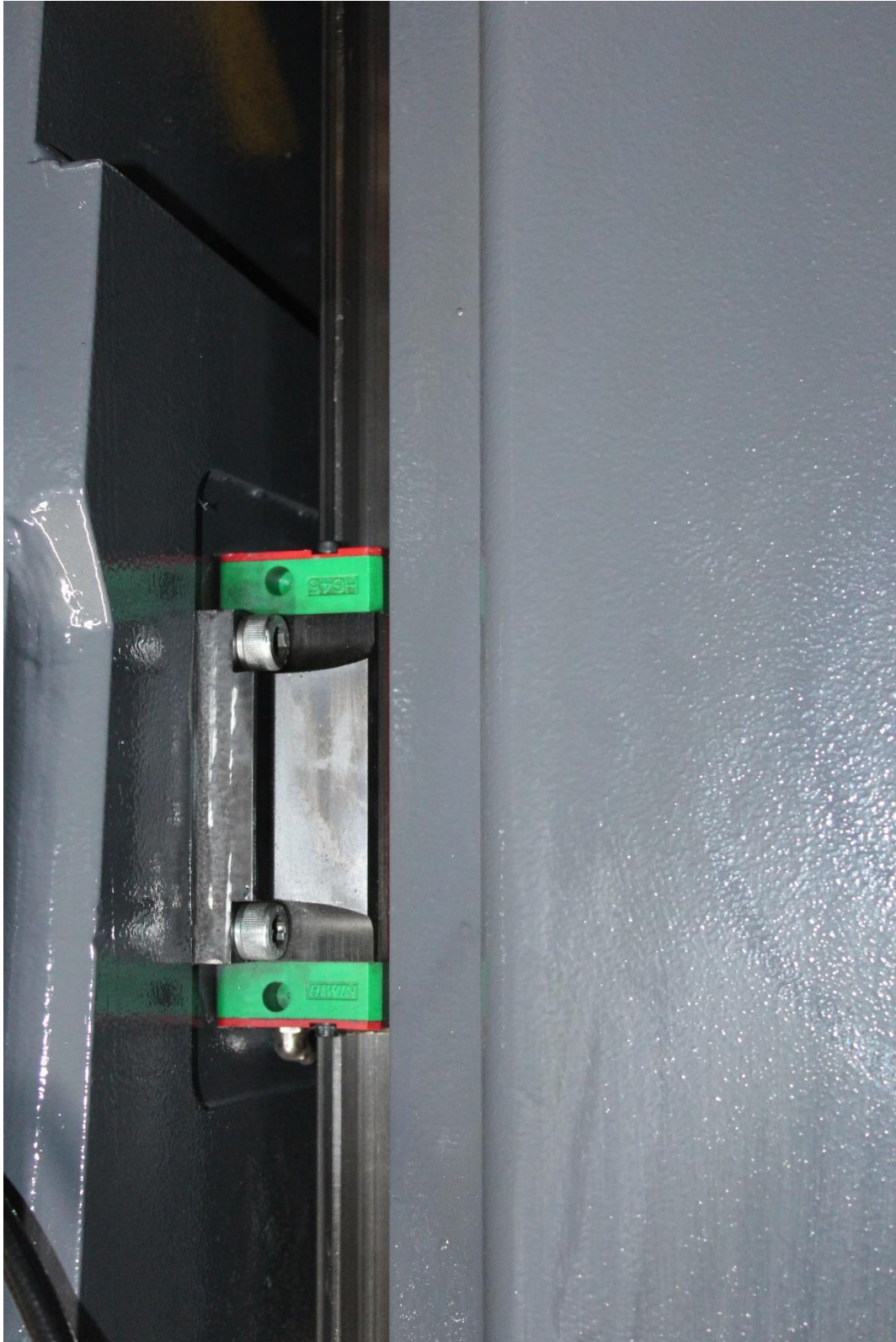
LINEAR SLIDES FOR BODY MOVING UP AND DOWN
