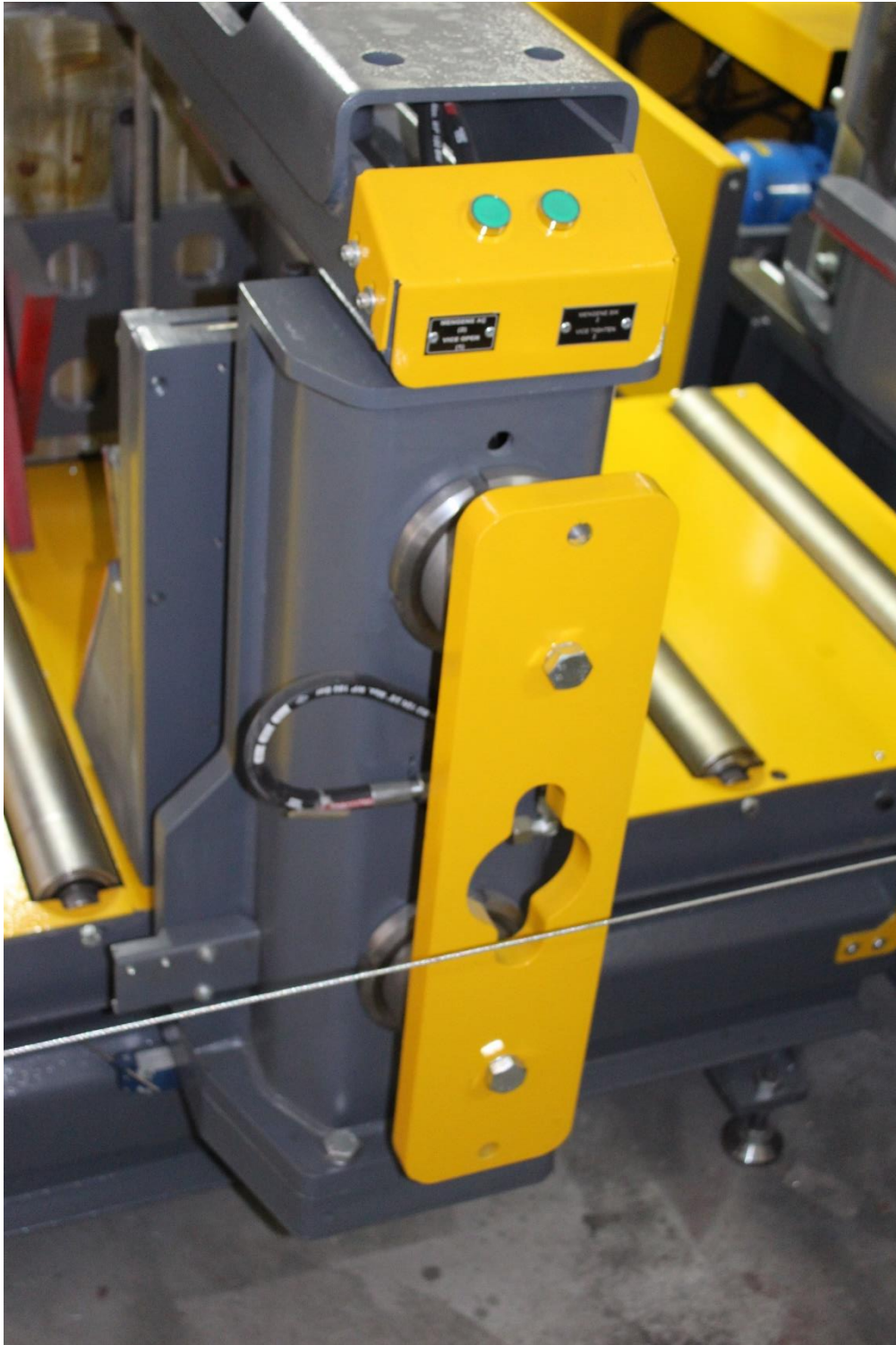
CONTROL BUTTONS ON FEEDING VICE FOR EASY USE.
