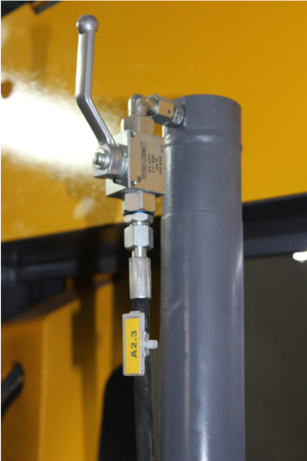
HYDRAULIC VALVE TO CLOSE/OPEN UPPER CLAMP
