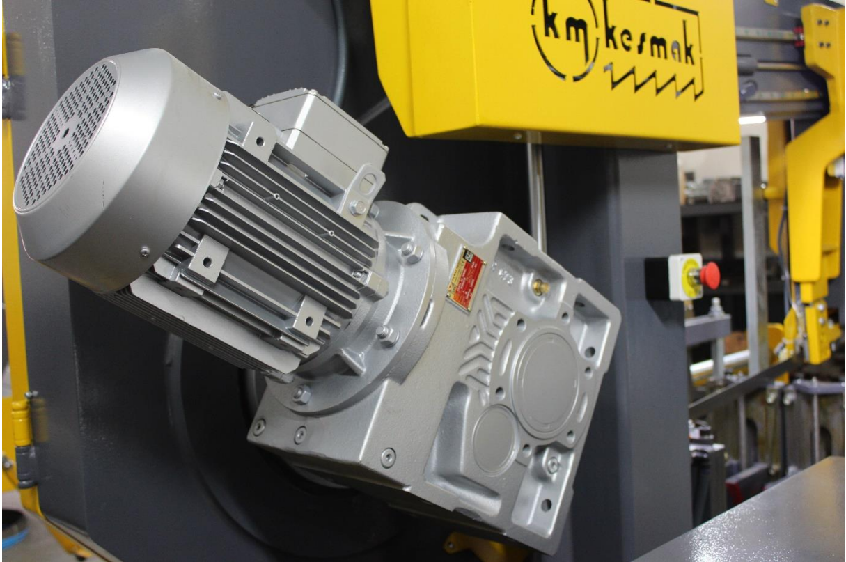
4 KW POWERED MOTOR WITH GEARBOX
