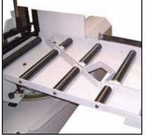
Connection element between machine and rolling table for unloading side. When using the machine for straight cut, the element is made by two part (as in the attacched picture). If it's required to cut angles, one of the two supporting pieces byt me removed to reduce the supported area so that the sawframe could rotate.
