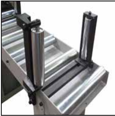
Pair of vertical steel containment rollers.(OPTIONAL)
